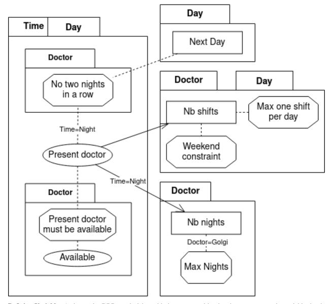
**Defining Variables** As in regular DRDs, a decision table is represented by drawing an arrow to the variable that is defined by the table from each of the other variables that appear in the table. However, in cDMN this does not mean that the table can only be used to compute the defined variable. It does not imply a computing order, but rather an order of defining.
